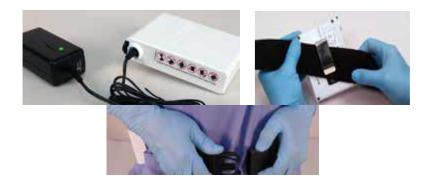
j. Assemble the battery onto the belt. Place the top edge of the Belt under the Battery Clip. Move the Belt fully under and up to the top of the Clip.
