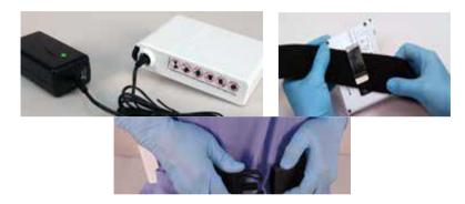
j. Assemble the battery onto the belt. Place the top edge of the Belt under the Battery Clip. Move the Belt fully under and up to the top of the Clip.
