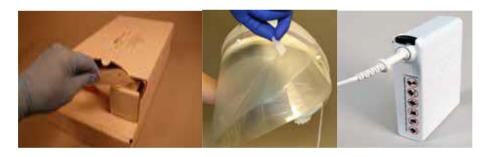
k. Connect the Helmet Power Cord to the Battery. Push the Power Cord Connector into the Battery Receptacle until the Secure Connection audibly clicks.
